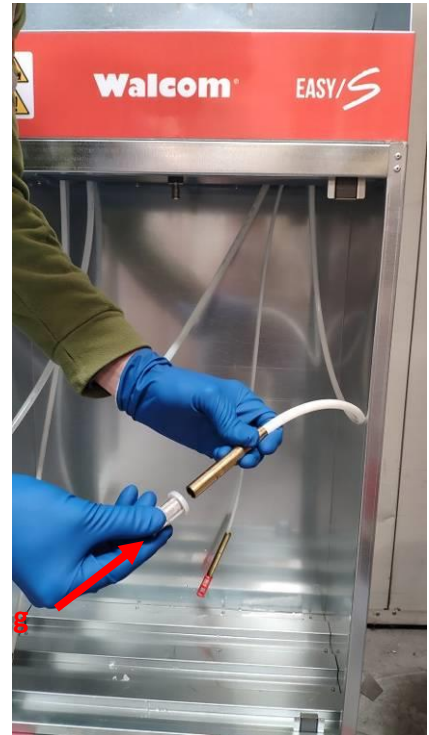
fig. 7.3. filter (g) CLEAN SOLVENT FLOW
