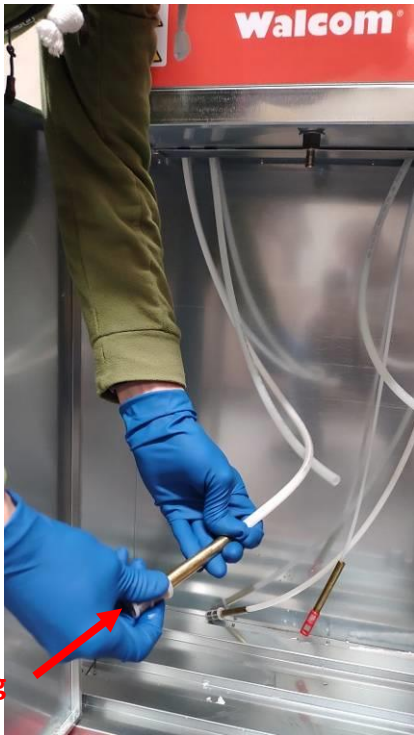
fig. 7.1. filter (g) RECYCLED SOLVENT FLOW
